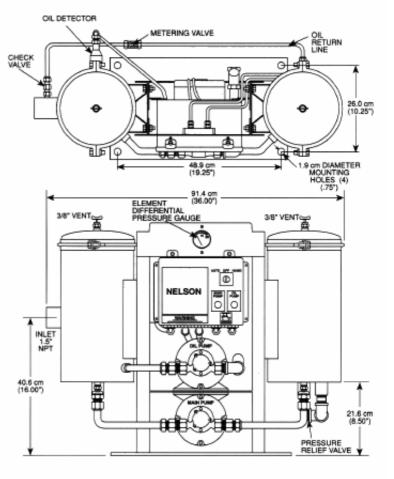
BB00311DXX 25GPM Separator Shown
